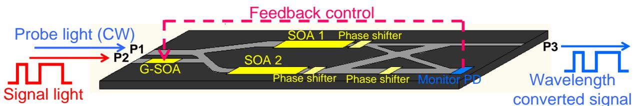
Figure 1. Schematic diagram of SOA-MZI wavelength converter monolithically integrated with a monitor PD and a gain control SOA
