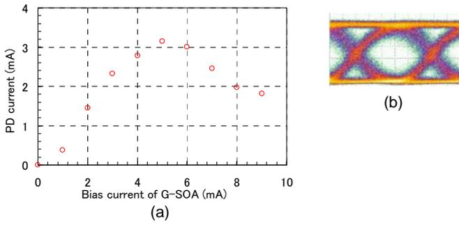
Figure 4. (a) Monitor PD current versus bias current of G-SOA. (b) The eye diagram of converted signal at the maximum monitor PD current.
