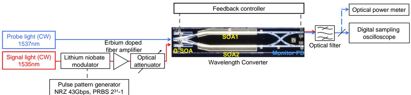
Figure 3. Schematic diagram of experimental setup.
