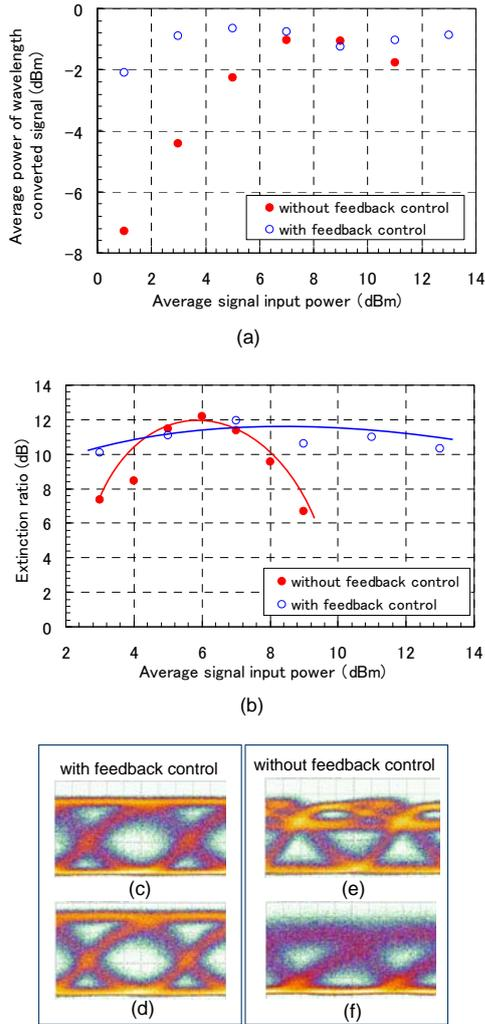
Figure 5. Characteristics of average power of wavelength converted signal and extinction ratio as well as eye diagrams of converted light. (a) Average power of wavelength converted signal as a function of average signal input power. (b) Extinction ratio versus average signal input power. (c) (d) Eye diagrams with feedback control in the power of +13 dBm and +3dBm, respectively. (e) and (f) Eye diagrams without feedback control in the power of +9dBm and +3dBm, respectively.
