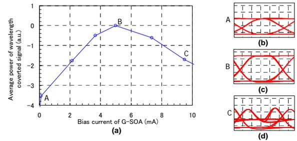
Figure 2. Characteristics of average power of wavelength converted signal and eye diagrams for 43Gbps NRZ signal. (a) Calculated average power of wavelength converted signal as a function of bias current of G-SOA. (b) The eye diagram at the point of A. (c) The eye diagram at the point of B. (d) The eye diagram at the point of C.
