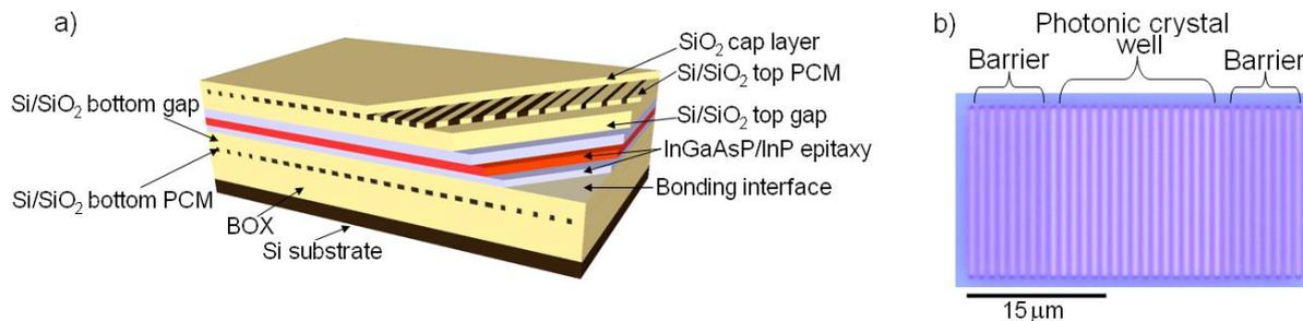
CMOS-compatible VCSELs using double photonic crystal mirrors: schematic view (a) and top SEM view (b) (see [21])
