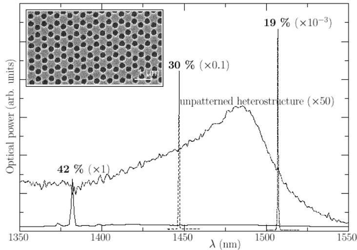
Low threshold, room temperature vertical emitting laser based on an InP two-dimensional photonic crystal membrane (graphite lattice): laser emission spectra for various air hole filling factors. A SEM top view of the structures is shown in the inset (see [15]).
