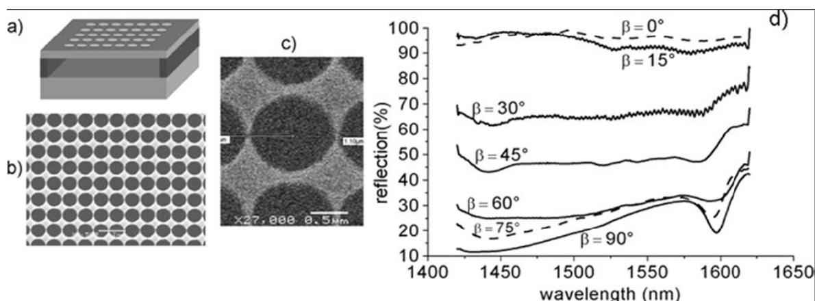
(a) Schematic representation of broadband and compact 2-D Photonic Crystal reflector. (b) SEM general view. (c) SEM close-up view of one cell of the lattice. (d) Experimental reflectivity spectra of the square lattice with elliptical holes, for various angles of polarization of the incident wave (see [14]).
