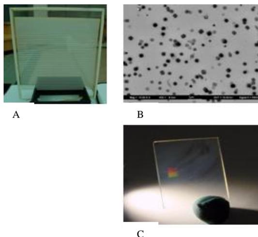
Figure 2 NaF-based glasses. (A) opaque pattern, (B) fine grain particles leading to transparency, (C) hologram made from B-type samples.
