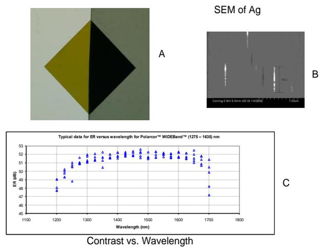
Figure 6 Polarizing glass; (A) visual contrast, (B) SEM of elongated silver particles
