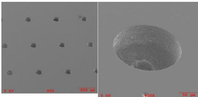
Figure 3 Example of photo-machinable Fotoform™.
