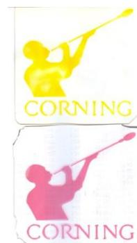
Figure 1. Example of Ag-based (top) and Au-based photosensitive glasses
