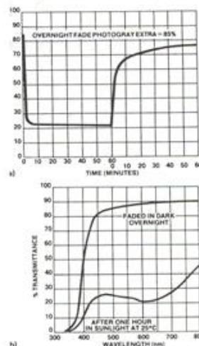
Figure 5 Example of darkening and fading of a photochromic glass.
