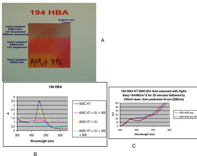
Figure 8 Examples of the photo-adaptive behavior, (A) color change as noted and described in text, (B) corresponding absorption spectra for the conditions noted, (C) evidence of dichroic behavior when bleached.
