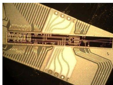
**Fig. 3:** Integrated tunable transmitter providing 4x28Gbit/s channels with grid-tuning.
