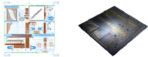
**Fig. 4:** Sample designs in the JePPIX process: mask layout (left) and finished multi-project wafer cell (right).
