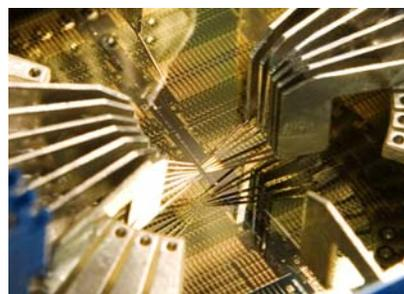
**Fig. 1:** Integrated InP DSDBR tunable laser-Mach Zehnder modulator devices undergoing on-wafer test
