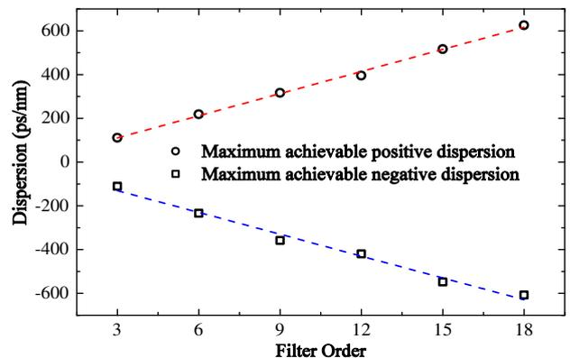
Fig. 2. Relation of attainable dispersion from a filter comprising  $M$ -port MMI couplers vs the filter order.
