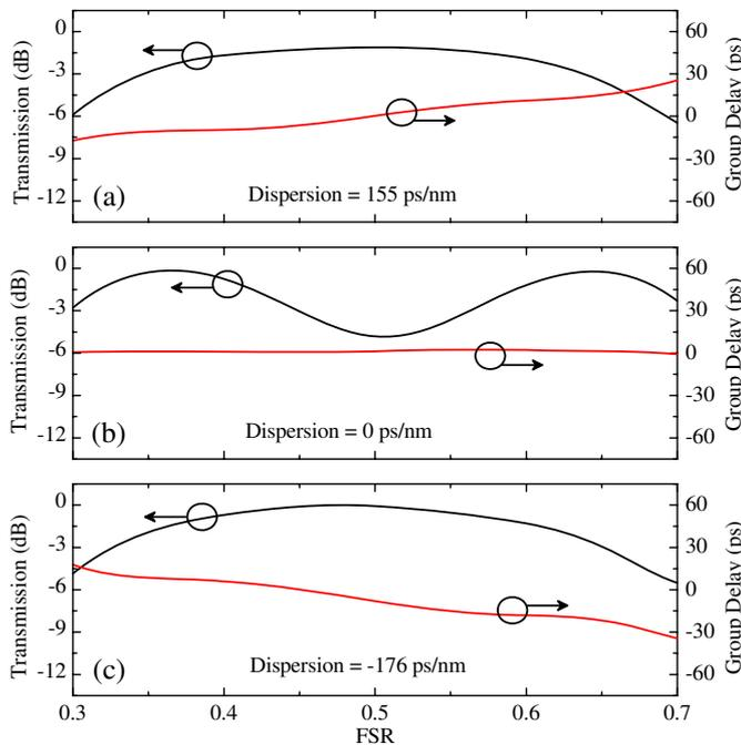
Fig. 3. Measured transmission (solid, black) and group delay slope (solid, red). Fraction of the filter  $FSR$  with positive (a), zero (b) and negative (c) dispersion for the fabricated filter.
