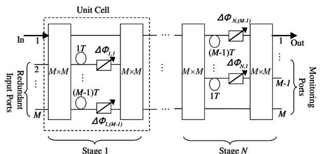
Fig. 1. Waveguide layout of a generalized filter comprising  $M$ -port MMI couplers. A single stage is shown in the dotted section. Ports with arrows are for input and output. Other ports are either redundant or used for monitoring purpose.
