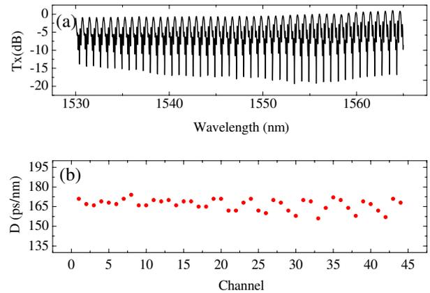
Fig. 4. (a) Measured transmission over a bandwidth of 35 nm (44 WDM channels) in the C-band, (b) Variation in filter dispersion for group delay ripple of less than  $\pm 5$  ps with more than 40% of filter  $FSR$  with linear group delay.
