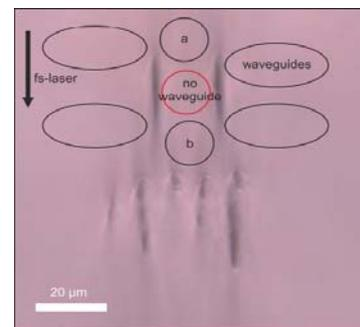
Figure 1 Bright-field microscope image of the end facet of the crystal where a pair of tracks with a distance of 18  $\mu\text{m}$  was written.
