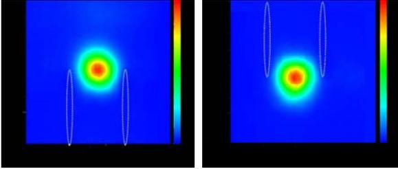
Figure 2. Near field intensity distribution at 633 nm for the two waveguides, a and b, in Fig. 1. The tracks are indicated by white dotted lines.
