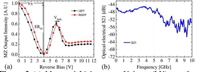
**Figure 3** (a) Measured Light versus Voltage (LV) transfer function (alternate arm at 0V); (b) Small signal optical-electrical S21 for the integrated laser-modulator formed photonic link.
