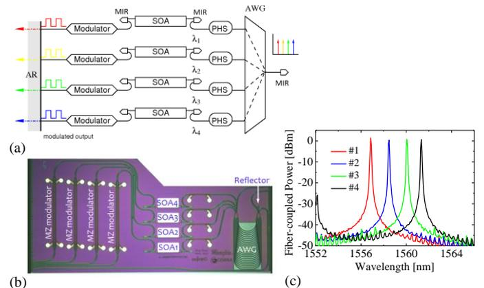
**Figure 1** (a) Schematic of the 4-channel transmitter device and (b) Microscope photograph of the realized device. The chip dimension is 2×4 mm<sup>2</sup>. (c) Superimposed lasing spectra of the four lasers channels.
