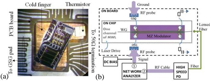
**Figure 2** (a) Microscope photograph top view of the transmitter wire bonded with testing board; (b) Schematic for one channel transmitter connection in the photonic link measurement setup.
