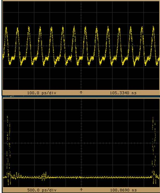
Figure 2. Sampling oscilloscope traces of modulated pulse trains at repetition rates of 14 GHz and 219 MHz. The double pulses at 219 MHz result from the limited bandwidth of the pattern generator.
