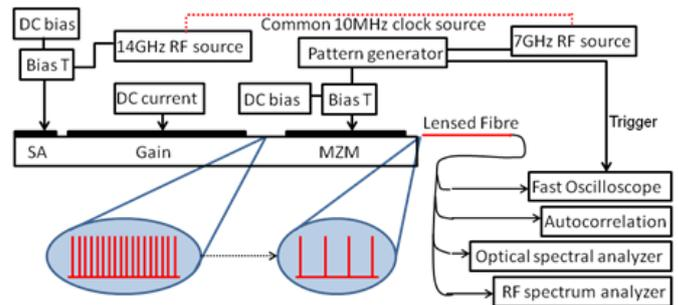
Figure 1. A schematic diagram of the integrated device and of the drive electronics used for hybrid modelocking and modulation of the pulse train, along with the associated characterization equipment.
