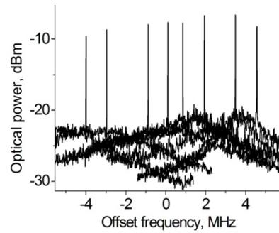
Figure 3. RF spectra of the fundamentally mode-locked laser at eight different hybrid modelocking frequencies, showing a continuous tuning range greater than 8 MHz.
