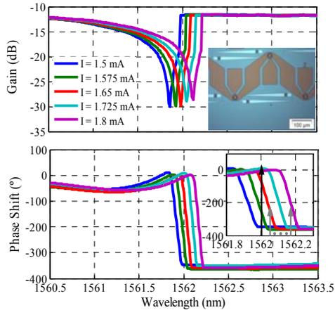
Fig. 2. Gain and phase transfer functions with the injection current.
