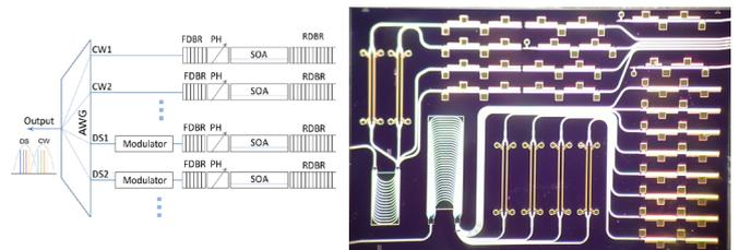
Figure 1. Schematic of the transmitter (left) and the photograph (right) of the fabricated devices. The size of the chip is only 4 mm x 6 mm.
