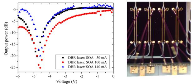
Fig. 4. Measured extinction ratio of 1 mm long MZM while changing the current injected to the SOA of the DBR laser (left). The photograph of wire-bonded modulators (right).
