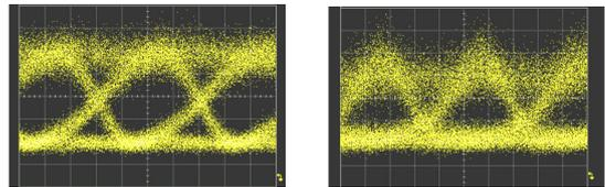
Fig. 5. Detected eye-diagrams at 12.5 Gbps of the MZM in B2B (left) and after transmission through 20 km long SMF (right).
