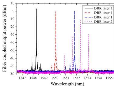
Fig. 2. Emission spectra measured for the 4-channel transmitter. The wavelength generated by the DBR laser no 2 was not properly tuned to the center of the AWG passband, which can be noticed on the spectrum.
