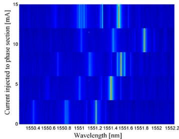
Fig. 3. The fine tuning of the DBR laser no 1 while biasing the SOA with 60 mA and changing the current injected to the PH. The source can be adjusted to the required wavelength, within the AWG passband by proper bias of the PH element. DBR mirrors remain unbiased for the experiment.
