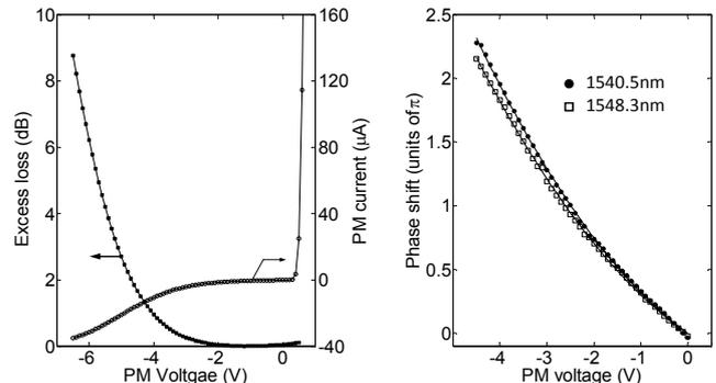
Fig.3. Induced excess loss (dB, left axis) and current through the phase shifter ( $\mu\text{A}$ , right axis) vs. applied PM Voltage (V).
