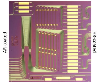
Fig. 1. Microscope image of the realized 6×6mm<sup>2</sup> pulse shaper chip.
