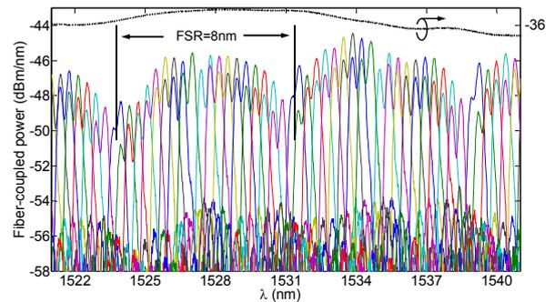
Fig.2. Fiber-coupled optical spectral power measured at input/output waveguides. The SOA in channel 11 is biased at 30mA; generated ASE is shown (dotted curve, right axis).
