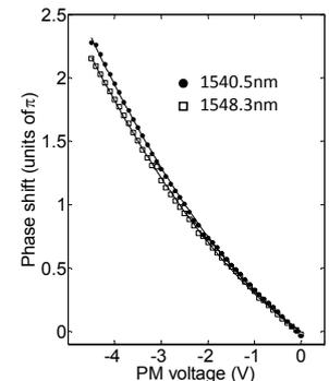
Fig.4. Measured phase shift (circles at  $\lambda=1540.5\text{nm}$ , open squares at  $\lambda=1548.3\text{nm}$ ) and quadratic polynomial fitted curve (solid line).
