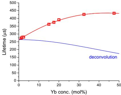
Figure 3.  $^2F_{5/2}$  lifetime as a function of  $\text{Yb}^{3+}$  concentration. The red line is the fit with the equation given in [5], while the blue line is the deconvolution of the fit that shows the self-quenching contribution.
