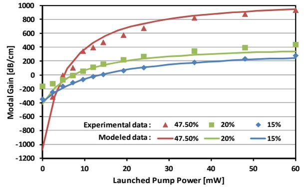
Figure 4. Waveguide modal gain at 981 nm versus launched pump power for different  $\text{Yb}^{3+}$  concentrations.
