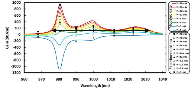
Figure 5. Waveguide modal gain for an  $\text{Yb}^{3+}$  concentration of 47.5% and different launched pump powers, calculated (lines) and measured (symbols); indication (arrow) of the spectral range of 55 nm with  $g_{mod} > 150 \text{ dB/cm}$ .
