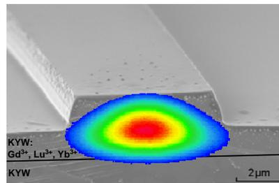
Figure 2. Cross-section of a channel waveguide prior to KY(WO<sub>4</sub>)<sub>2</sub> overgrowth.
