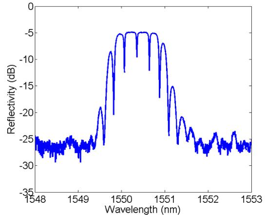
Figure 3 The Fabry-Perot Bragg grating signature of a 5mm cantilever device.
