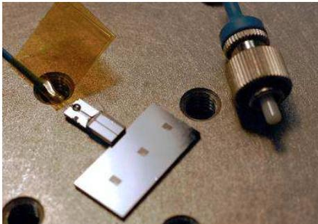
Figure 2 Photograph of three micro-membrane structures integrated into a single optical chip.
