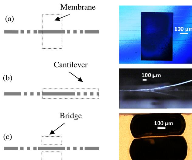
Figure 1 Images of the three micromechanical integrated optical components developed, indicating waveguide (thick grey) Bragg grating (dashed grey) and micro-mechanical component (thin black dashed line), for (a) micro-membrane (b) micro-cantilever (c) micro-bridge.
