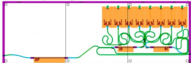
Figure 2. Mask layout of the 8:1 integrated optical serializer
