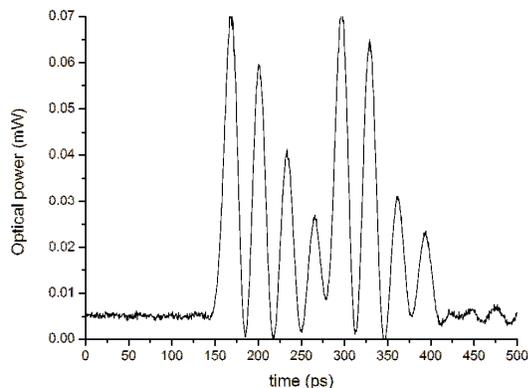
Figure 3. Pulse response of the 8:1 serializer circuit
