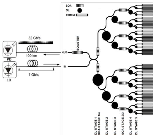
Figure 1. Schematic of the read-out system
