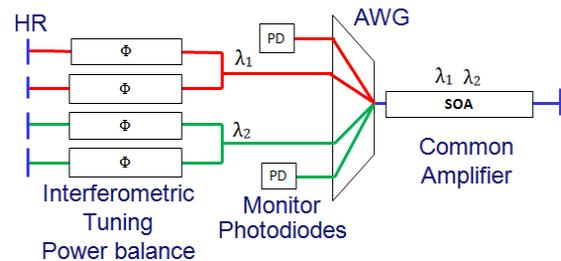
Fig.1. Schematic of the linear AWG-based laser.
