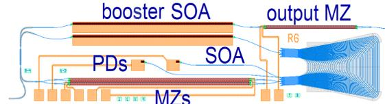
Fig.4. Mask layout of the linear AWG-based laser.
