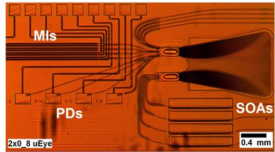
Fig.3. Picture of the linear dual-wavelength AWG-laser.
