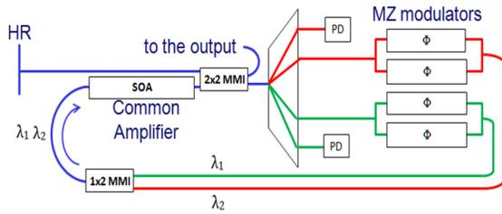
Fig.2. Schematic of the ring AWG-based laser.
