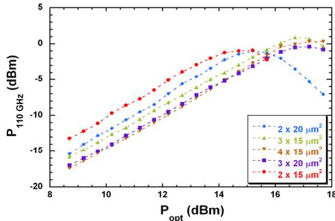
Figure 3: Power saturation at 110 GHz for various UTC-PDs with different active area dimensions. The reverse bias voltage was 3 V.
