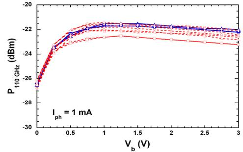
Figure 4: Generated power at 110 GHz for straight (blue) and angled (red) UTC-PDs.
