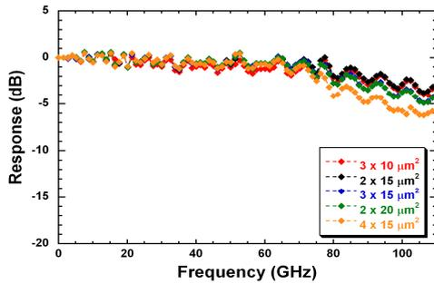
Figure 2: Frequency response up to 110 GHz from UTC-PDs with various active area dimensions.
