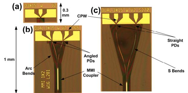
Figure 1: Images of chips with (a) Single UTC-PDs, (b) Dual angled UTC-PDs with Arc-Type bends and (c) Dual straight UTC-PDs with S-type bends.
