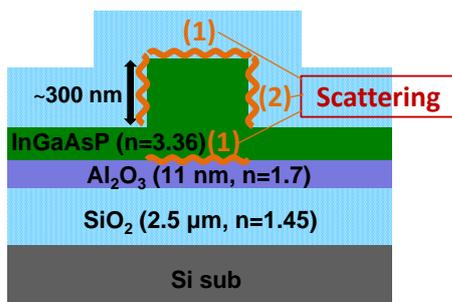
Fig. 1 Scattering of InGaAsP photonic-wire waveguide.
