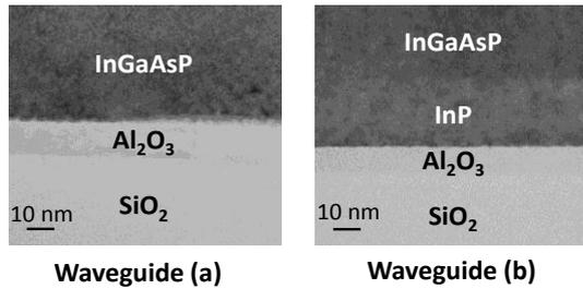
Fig. 4 TEM images of the bonded interfaces of the waveguide (a) and (b).
