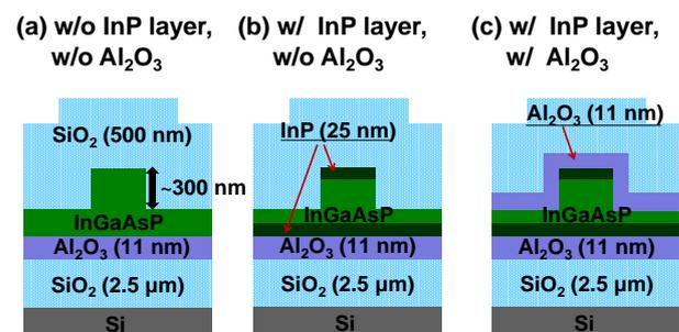
Fig. 2 Schematics of three types of fabricated waveguides.
