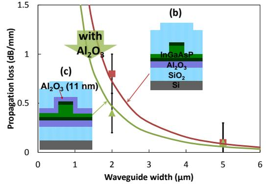
Fig. 5 Propagation losses of the waveguides (b) without Al<sub>2</sub>O<sub>3</sub> passivation and the waveguide (c) with Al<sub>2</sub>O<sub>3</sub> passivation
