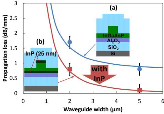
Fig. 3 Propagation losses of the waveguides (a) without InP passivation and the waveguide (b) with InP passivation.
