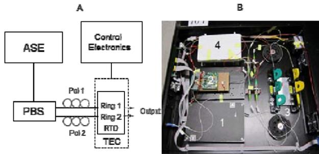
**Figure 1** Fabricated portable frequency comb device. A) Schematic of the device where the frequency comb is generated from the micro-ring resonator response by the ASE excitation. B) A photograph of the frequency comb where 1 – ASE source, 2 – micro-ring resonator device, TEC and control electronic, 3 – polarization controller, 4 – PBS and fiber management.
