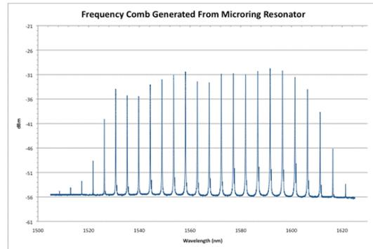
**Figure 2** Frequency Comb signal from the resonator-based Er-doped ASE device. The comb effectively spans both the C and L band, and can be tuned for increased flatness via two LD pump diodes.
