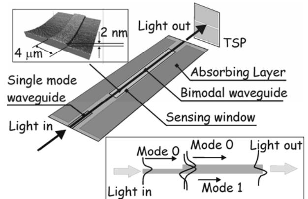
Figure 1. Sketch of the device. Top inset: an AFM image of the ridge designed for single mode operation of the waveguide in lateral direction. Inset below: the principle of mode splitting is sketched.
