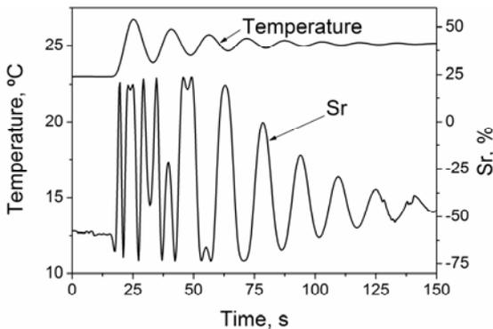
Figure 2. Response of the sensor to the temperature changes
