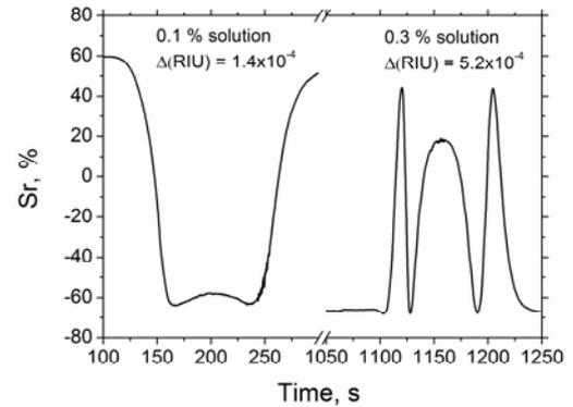
Figure 3. Response of the sensor to injection of glycerin solutions with concentrations of 0.1 % and 0.3 % (both by volume)
