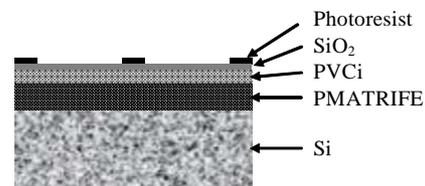
Figure 1. Representation of different layers before photolithography step
