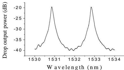
Figure 4. Drop output power with 1 nm step wavelength
