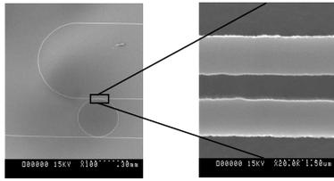
Figure 2. SEM photos of PVCi etched structure
