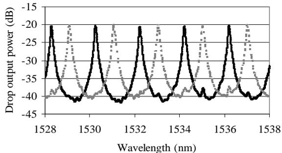
Figure 3. Drop output power with 2.5 nm step wavelength (TE / TM)
