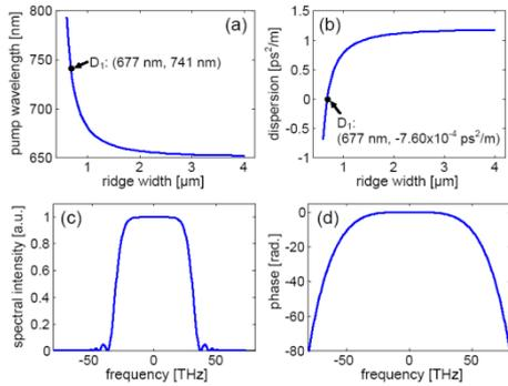
Figure 2. (a) Pump wavelength versus ridge width. (b) Signal group velocity dispersion versus ridge width. (c) Normalized joint spectral intensity  $|\Phi|^2$  with a FWHM bandwidth of  $\sim 61$  THz ( $\sim 456$  nm). (d) Phase of the spectral amplitude.
