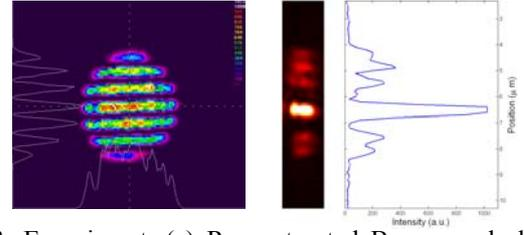
Figure 3. Experiment. (a) Reconstructed Bragg mode before the input coupling stage using an SLM. (b) Profile of the pump mode at the output facet of the waveguide along with the transverse intensity profile.
