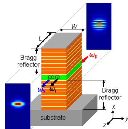
Figure 1. Schematic of a typical BRW with intensity profiles of the pump  $\omega_p$  and of the downconverted photons  $\omega_s$  and  $\omega_i$ .
