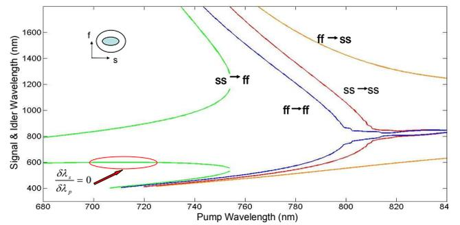
Figure 2. Phasematching curve for a birefringent fibre, with pairs annihilated and created in the fast (ff) and slow (ss) axis, respectively.
