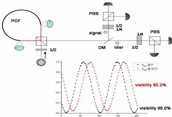
Figure 3. Setup of the entangled photon pair source.
