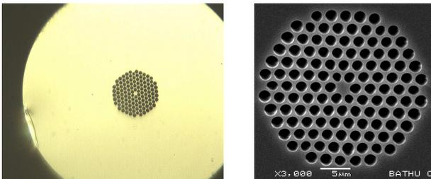
Figure 1. Profile of a nanostructured Photonic Crystal Fibre.
