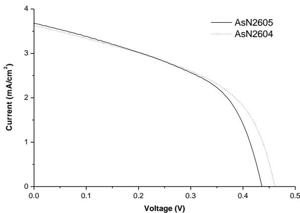
Figure 2: A graph showing the AM1.5G I-V characteristics for the annealed (solid) and unannealed (dotted) structures
