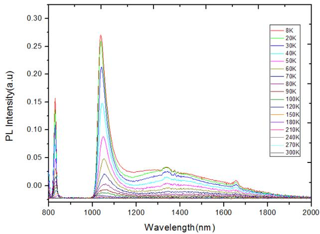
Figure 1: The photoluminescence results for the annealed structure.
