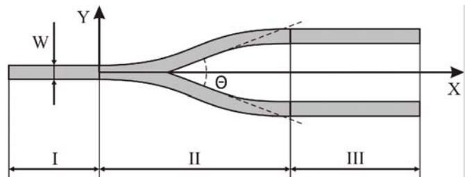
Figure 1. Layout of the Y-branching power divider.  $\Theta$  is branching angle,  $W$  is channel waveguide width.
