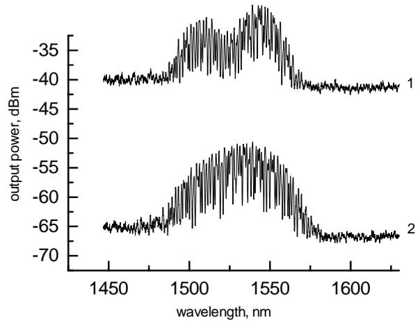
Figure 4. Spectral dependence of the power of IR radiation at output port of Y-branching power divider with cosine topology and the extra taper introduced in branching region (see Fig.3): (1)  $\Theta = 1.4^\circ$  and the extra taper has  $L_{et} = 130 \mu\text{m}$  and  $2w = 1.26 \mu\text{m}$ , (2)  $\Theta = 1.9^\circ$ ,  $L_{et} = 100 \mu\text{m}$  and  $2w = 1.18 \mu\text{m}$ . To escape overlapping, curve 2 is shifted for -24 dBm relative to curve 1.
