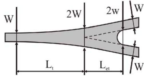
Figure 3. Topology of branching region:  $L_t$  – taper length,  $L_{et}$  and  $2w$  – length and width of extra taper. Dashed lines show Y-branching without extra taper.
