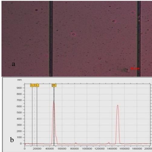
Figure 2. a. Microscopy image, b. height measurement of etched channels.
