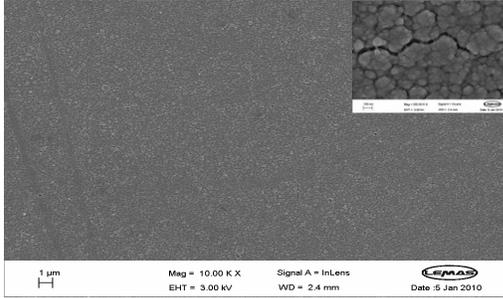
Figure 1. SEM image of the TWL film on silica. Inset showing image at higher magnification.
