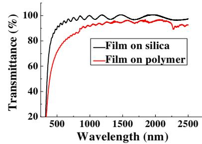
Figure 3. Transmittance of the glass film on silica and polymer substrates.
