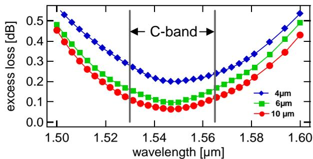
Fig.2 Excess Loss of  $2 \times 2$  MMI-coupler over wavelength around 1550nm and as function of  $W_{\text{MMI}}$ .
