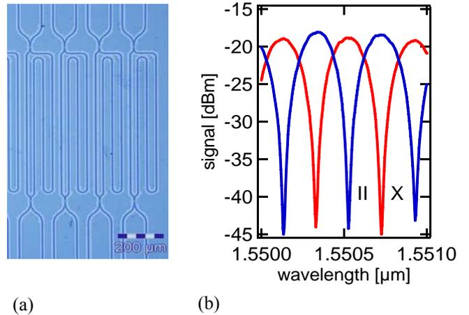
Fig.3 Realized  $2 \times 2$  Mach-Zehnder Interferometers with delay line of 25 ps (3 a) and measured transfer curve at 1550nm for TE-mode (3 b). Extinction ratios for bar and cross port exceed 20 dB.
