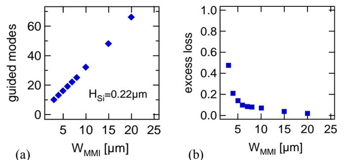
Fig.1a Relation between guided modes and width of multimode-section in silicon-on-insulator material with Si-thickness H of 0.22μm. Fig. 1b shows the excess loss of 2×2 MMI-coupler realized in the same substrate for TE-mode.
