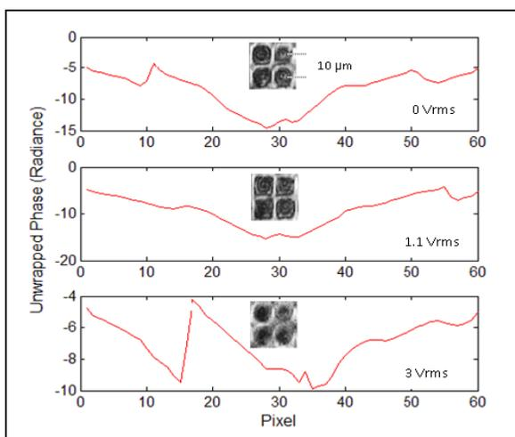
Figure:1 Interferograms of four lenslets along with unwrapped phase profile across one lenslet at  $0\text{Vrms}$ ,  $1.1\text{Vrms}$  and  $3\text{Vrms}$ . The phase profile is smooth and parabolic like at  $1.1\text{Vrms}$ .
