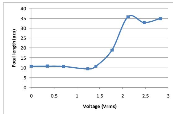
Figure:3 Focal length variation of one lenslet with respect to applied voltage.
