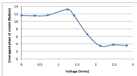
Figure:2 The variation of unwrapped phase of one lenslet with respect to applied voltage
