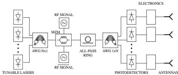
Fig. 2: Schematic of the integrated beamformer.
