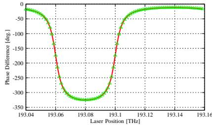
Fig. 3: Induced phase shift for a 40 GHz RF signal in one channel vs laser position in the ring FSR. The triangle symbols indicate the tunable laser discrete steps.
