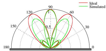
Fig. 4: Radiation diagram vs.  $\Theta$  [deg.] for a uniform linear 4 element array, for different  $\alpha$  values and  $d = \lambda/2$
