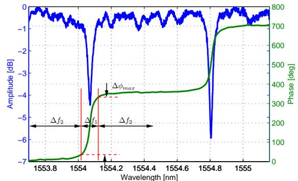
**Fig. 1:** Power transmission and phase characterization of an all-pass single RR in two FSRs.
