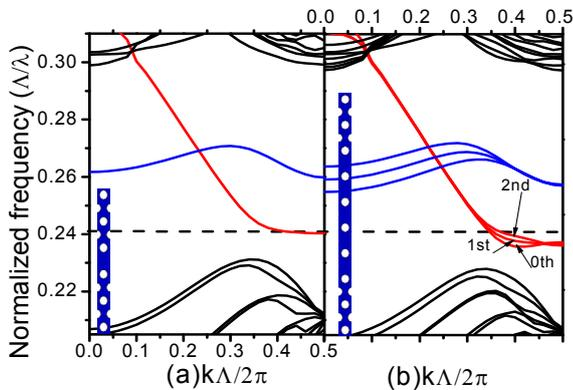
Figure 2. Dispersion diagram for TE polarization of the PhCWs calculated using 3D PWE method. The supercells are shown in the insets. Black lines are PhC modes. Red (blue) line are even (odd) gap-guided modes.
