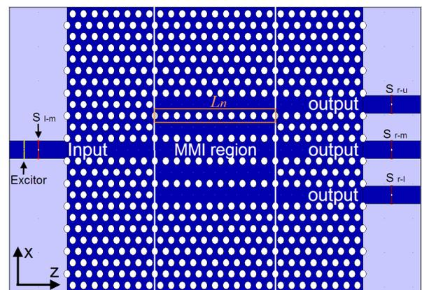
Figure 1. Schematic layout of 1x3 beam splitter consisting of input, MMI and output PhCWs, and excitor and sensors arranged in the ridge waveguides.
