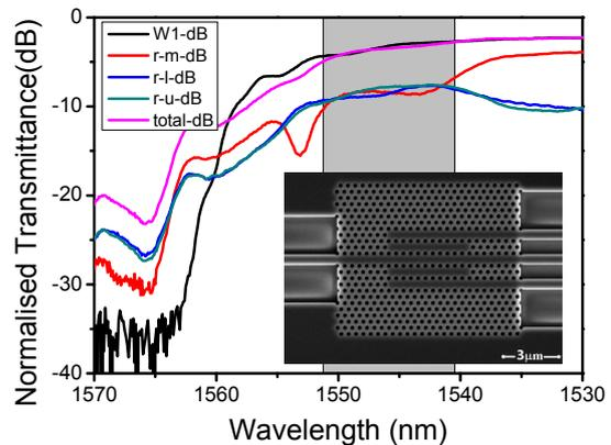
Figure 4. Measured normalised TE-polarized transmittance (dB) for the 1x3 splitter in Fig. 4, the inset is an SEM photograph of the component.
