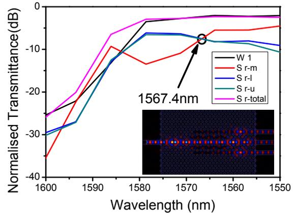
Figure 3. Normalised TE-polarized transmittance (dB) for the splitter with  $L_n=11\Lambda$ , simulated by 3D FDTD. The inset is a snapshot of  $H_y$  at 1567.4 nm.
