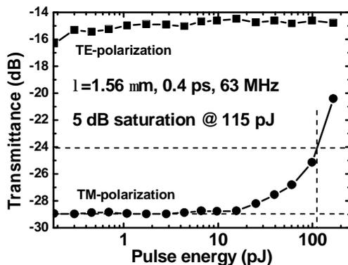
Figure 2. Transmittances of TE- and TM-polarized light as functions of input pulse energy.
