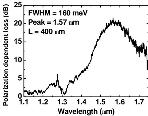
Figure 1. Polarization dependent loss defined by ratio of transmittances of TE- and TM-polarized light
