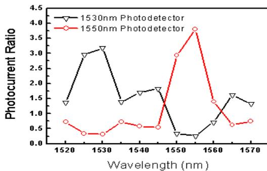
Figure 2. Response spectra measured from photodetectors.
