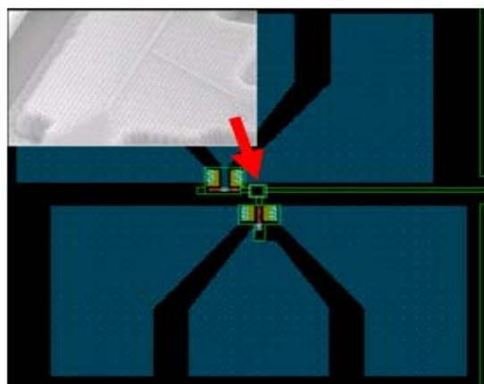
Figure 1. Layout of integrated nano-optics system. The inset is the PC demultiplexer.
