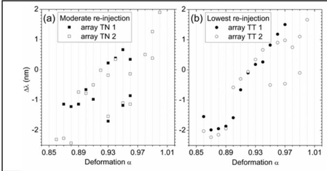
Figure 3. DFB laser arrays using affine deformation: evolution of the emission wavelength difference  $\Delta\lambda$ : (a) with one normal end introducing moderate level of feedback and (b) with two tilted ends ensuring lowest possible feedback.
