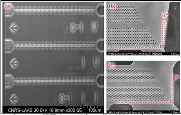
Figure 2. Array of DFB lasers: (a) 3 out of the 15 lasers of the array; (b) close-up on a tilted output mirror; (c) close-up on a normal output mirror.
