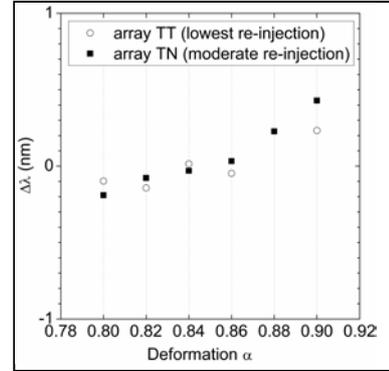
Figure 4. DFB laser arrays using double deformation: evolution of the relative emission wavelength with one normal end introducing moderate level of feedback (black squares) and with two tilted ends ensuring lowest possible feedback (white circles).
