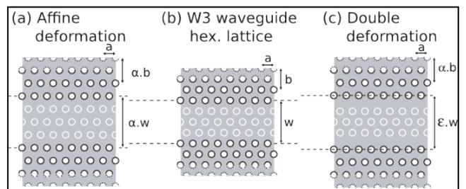
Figure 1. Geometry description: (b) undeformed W3 waveguide; (a) affine deformation; (c) double deformation
