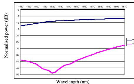
Fig. 4 Spectral characteristics of the polarization beam splitter at output 2 (transmitted). The blue curve indicates the TE polarization and the purple curve shows the TM polarization.
