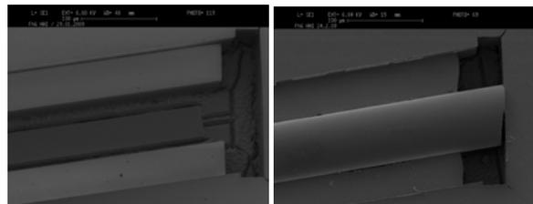
Fig. 1: SEM photos of U grooves with (right) and without (left) angled fiber inserted.
