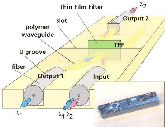
Fig. 2: The schematic of the 1X2 multiplexer
