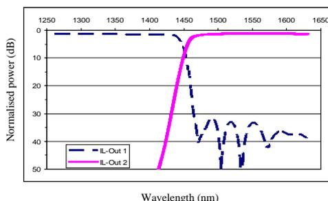
Fig. 3 Spectral characteristics of the 1X2 multiplexer, with the blue curve indicating the signal at output #1 (reflected) and the purple curve the signal at output #2 (transmitted).
