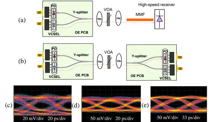
Figure 4. Link configurations when the optical transceiver is employed with: (a) an external optical component (high-speed fiber-coupled receiver) and corresponding received eye diagrams for (c) transmit and (d) receive operation mode at 10 Gb/s, and (b) in a link configuration with (e) corresponding received eye diagram at 6 Gb/s.
