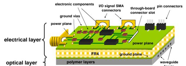
Figure 1. Schematic of OE PCB with various features noted.
