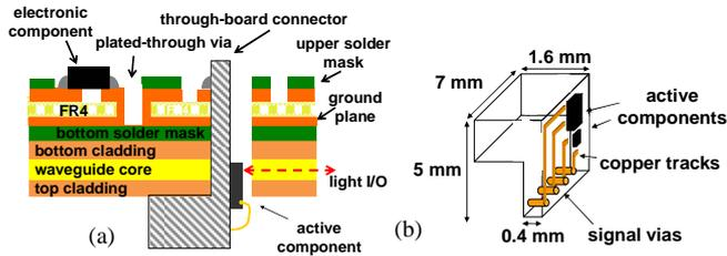
Figure 2. (a) Cross section of realised OE PCB with fitted electro-optic connector and (b) schematic of the L-connector with dimensions noted.
