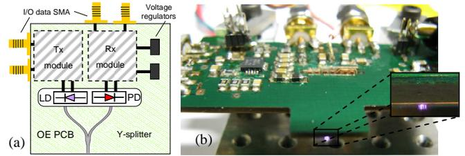
Figure 3. (a) Schematic of realised optical transceiver and (b) photograph of the actual unit with inset picture of illuminated output waveguide facet.
