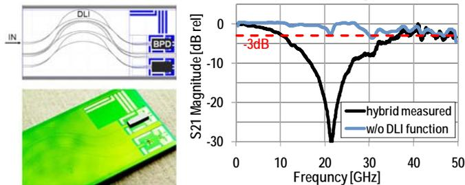
Fig 1a: DPSK receiver board. Fig. 1b: S<sub>21</sub> characteristics of the assembly and calculated o/e bandwidth.
