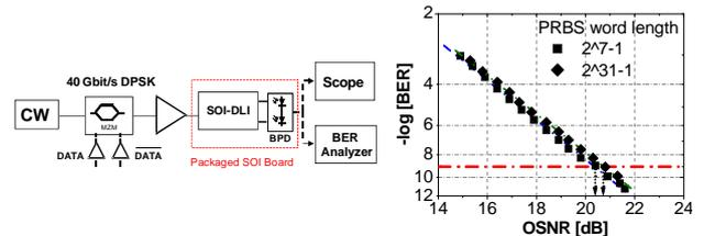
Fig. 3a: Test-bed for 40 Gbps non-return to zero (NRZ) DPSK, Fig. 3b: BER vs. OSNR for pseudo random bit sequences (PRBS) with word lengths of  $2^7-1$  and  $2^{31}-1$ .
