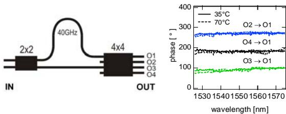
Fig. 2a: Layout of a 4x4 MMI test structure and Fig. 2b: results of phase measurements.
