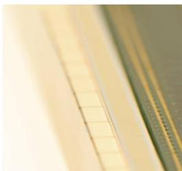
Figure 3. Part of a super array assembled using monolithic lasers containing 16 elements.
