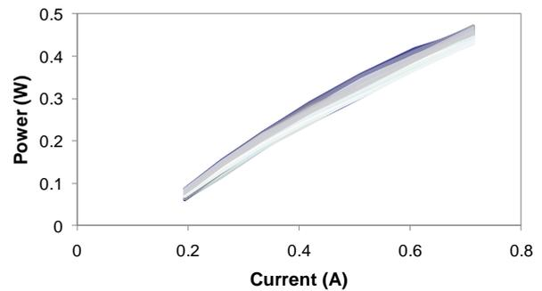
Figure 4. Light-current characteristics of 250 elements of a 980 nm super array.
