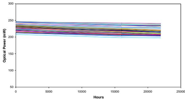
Figure 2. 22,000 hour lifetest of 64 element 200 mW, 8xx nm single mode laser module.
