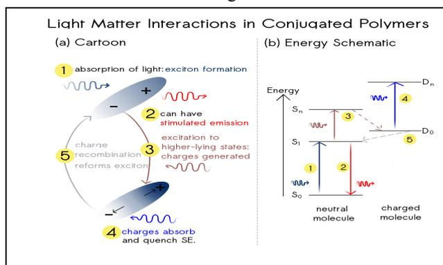
Figure 1. Schematic showing light-matter interactions in conjugated polymers. (a) Cartoon, (b) Energy Level Schematic demonstrating (1) absorption of light ( $S_0 \rightarrow S_1$ ) and formation of exciton, (2) stimulated emission (SE), (3) re-excitation to  $S_n$ , to form charges ( $D_n$ ) (4) absorption by the charges (which overlaps spectrally with SE) and (5) recombination of the charges to form an exciton ( $S_1$ ) and recovery of the stimulated emission.)
