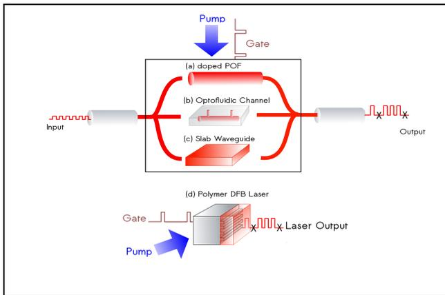
Figure 3. Schematic showing photonic devices using ultrafast switching (a) doped plastic optical fiber (POF), (b) optofluidic channel, (c) slab waveguide and (d) polymer distributed feedback (DFB) laser.
