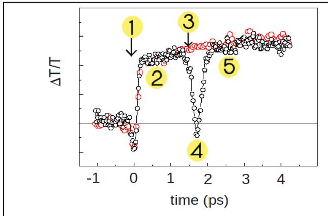
Figure 2. Pump-probe (red) and pump-push-probe (black) dynamics of polyfluorene-doped POF.
