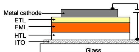
Figure 1: Schematic of the multilayer organic light-emitting device with the ITO as bottom electrode. EML is the emissive layer, ETL the electron transport layer and HTL the hole transport layer, all layers being organic.
