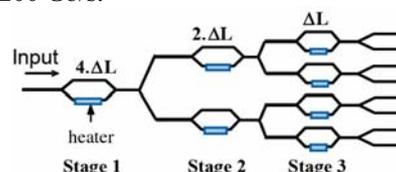
Figure 2: Schematic of the 8 channel DEMUX based on asymmetric MZIs;  $4\Delta L=97.2$   $\mu\text{m}$  for  $\Delta\lambda=3.2$  nm around 1550 nm, where  $a\Delta L$  and  $\Delta\lambda$  are the length difference between two arms of the asymmetric MZIs and optical channel spacing, respectively.
