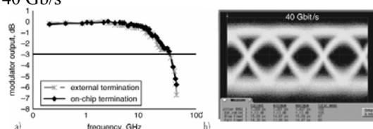
Figure 1: a) Represent the response of the modulator as a function of the RF frequency for a 1 mm active area. (b) Optical eye diagram of the modulator with a 1 mm long active area [2]
