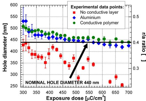
Figure 1. Experimental values of hole diameter and corresponding radius to lattice period ( $r/a$ ) ratio against electron-beam lithography exposure dose, for three different exposure conditions: without any conductive layer (square points), with 40-nm-thick Al layer used (rhombus points) and 100-nm-thick PEDOT:PSS layer used (circle points).
