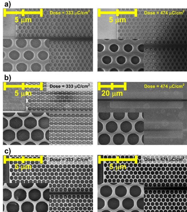
Figure 2. SEM micrographs of overall photonic crystal lattice and hole shape evolution in HSQ resist for doses of 333 and 474  $\mu\text{C}/\text{cm}^2$  and different exposure conditions: a) exposure without any conductive layer; b) 40-nm-thick Al layer used; c) 100-nm-thick PEDOT:PSS conductive polymer layer used.
