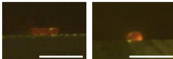
Figure 1. Unmelted and melted waveguides. The unmelted waveguide on the left (annealed at  $230^\circ\text{C}$ ) retains its rectangular cross-section whereas the waveguide on the right, annealed at  $290^\circ\text{C}$ , has a hemispherical cross-section.
