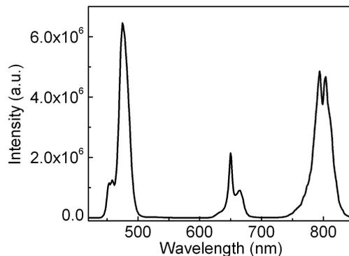
Fig. 1 The ASE upconversion emission spectra of Tm<sup>3+</sup>/Yb<sup>3+</sup> co-doped NMAG glass channel waveguides under 980nm wavelength laser diode excitation.
