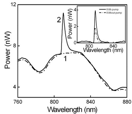
Fig.2 OSA spectra recorded from the output end-facet of 2.2 cm long  $Tm^{3+}/Yb^{3+}$  co-doped NMAG glass waveguide amplifier. Curve 1: Amplified spontaneous emission (ASE). Curve 2: ASE together with amplified 810nm signal under 457mW 980nm wavelength laser diode excitation. Inset: 810nm signal without pumping and with 457mW 980nm laser pumping with removal of ASE.
