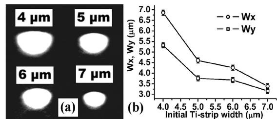
Fig. 1 (a) Near-field TM mode patterns of NS Ti:Mg:Er:LN strip waveguides at 1.5 $\mu$ m wavelength. (b) Mode size versus initial Ti-strip width.
