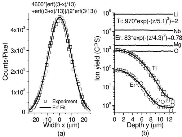
Fig. 2 (a) Surface <sup>48</sup>Ti profile and (b) depth profiles of <sup>7</sup>Li, <sup>93</sup>Nb, <sup>16</sup>O, <sup>24</sup>Mg, <sup>48</sup>Ti and <sup>166</sup>Er in 6- $\mu\text{m}$ -wide NS Ti:Mg:Er:LN strip waveguide
