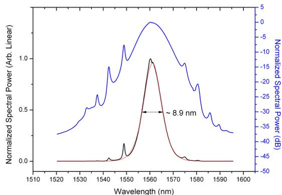
Figure 3. Optical spectrum of the modelocked waveguide laser, linear (Black) with  $\text{Sech}^2$  fit (Red), and logarithmic (Blue).
