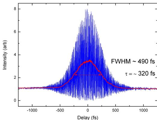
Figure 2. An interferometric autocorrelation of the output from the laser (Blue), with inferred intensity autocorrelation (Red).
