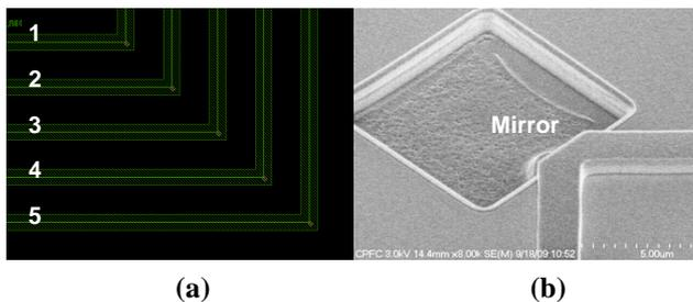
Figure 3: (a) Five corner turning mirror devices having five different mirror plane shifts and (b) the SEM image of a mirror
