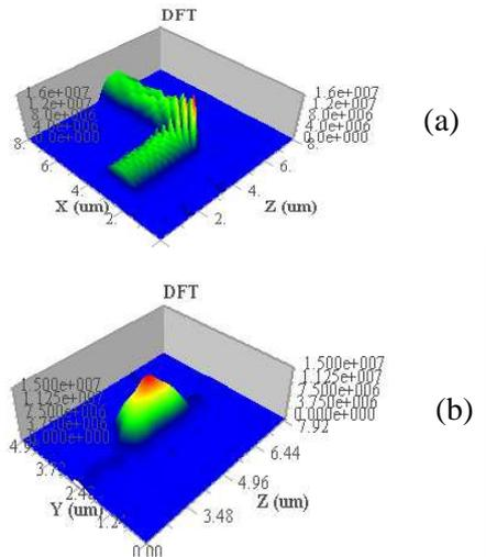
Figure 2: FDTD simulations with the selected corner mirror: (a) the propagation optical beam and (b) the output mode
