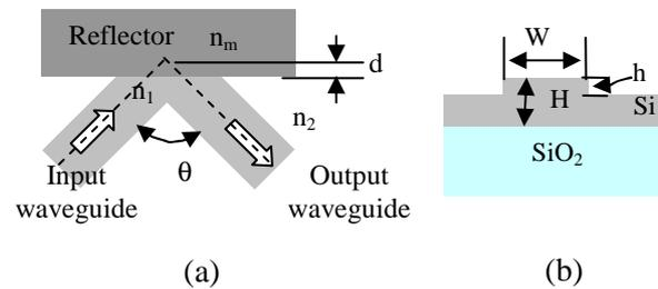
Figure 1: (a) Schematic geometry of SOI based corner mirror; (b) cross-sectional view of SOI rib waveguide
