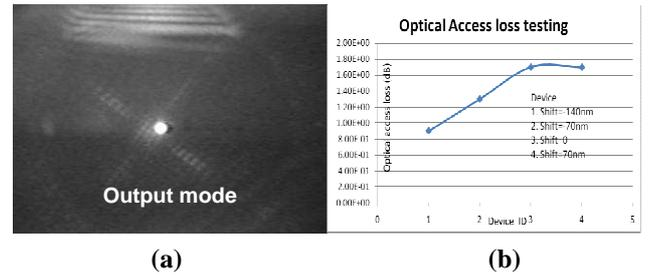
Figure 4: (a) an experimental optical guided-mode output and (b) the measured values of optical access loss for four devices
