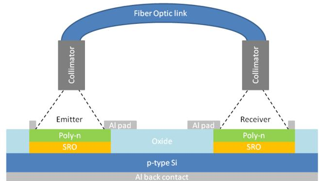
Figure 1. Scheme of the transceiver. Two identical devices are used as emitter and as receiver. The optical link is formed with an optical fiber.
