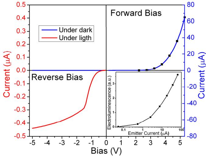
Figure 2. Current-Voltage characteristics under dark (blue) and under illumination (red). Black dots show current values at which EL signal (shown in the inset) was recorded. Left panel shows the photodetector region of the receiver.
