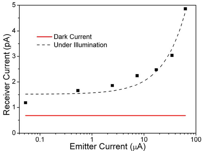
Figure 3. Photocurrent measured at the receiver versus the injected current at the source.
