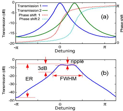
Figure 2. Principle of the bandwidth tunable filter. (a) Transmission and phase shift of the two microring resonators. (b) Characteristics of the bandwidth tunable filter. Here, we assume  $\kappa = 0.5, a = 0.99$ .
