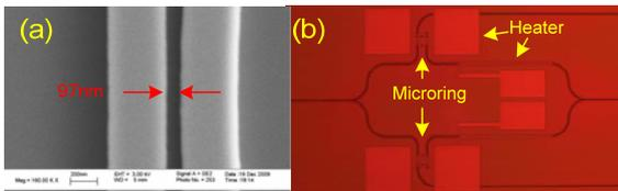
Figure 3. (a) Scanning electron microscope (SEM) top view image of the coupling region of the microring resonator. (b) Optical microscope picture of the fabricated device. Two identical add-drop microring resonators with micro-heaters are inserted in the two arms of the MZI structure. The straight sections of the two arms are also both implemented with heaters.
