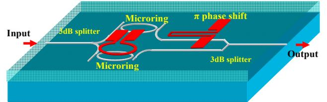
Figure 1. Structure of the microring-MZI bandwidth-tunable filter. It consists of two 3 dB splitters and two identical microring resonators. One heater is added on top of one microring resonator for resonance offset tuning. Another heater is added on top of one straight waveguide for phase tuning of the MZI.
