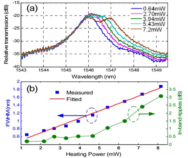
Figure 4. (a) Measured transmissions of the filter with different microring heating powers for the TE mode of the filter. (b) Measured bandwidth and in-band ripples versus microring heating power.
