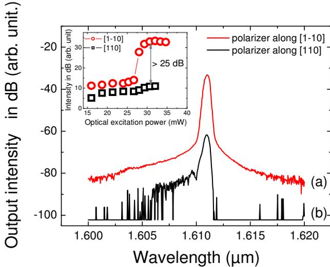
Figure 2 : RT CW laser emission spectra of a 3\*6 QDHs VCSEL as function of the polarizer orientation ( (a) along [1-10], (b) along [110]), at an excitation power of 30 mW. Inset represents the VCSEL light output integrated intensity versus the optical excitation power, depending on the direction axis of the polarizer, along [110] (squares) and along [1-10] (circles)
