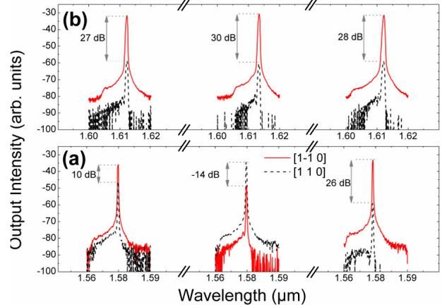
Figure 3 : Typical polarization resolved room temperature spectra from 3\*3 QW VCSELs (a) and 3\*6 QDH VCSELs (b), measured above threshold (in CW) at different location on samples (average spacing between VCSELs of 4 mm) Continuous line corresponds to the polarizer orientation along [1-10] direction, dashed lines along the [110]. Close to each spectra, the OPSR is indicated.
