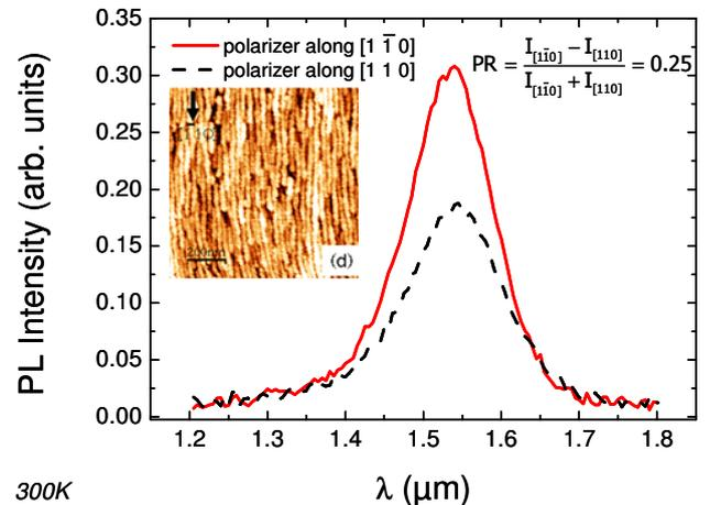
Figure 1 : RT PL of a six QDHs layers sample, separated with a GaInAsP spacer layer of 15nm, as function of the polarizer orientation (collinear with [110] or [1-10] direction). Inset is a  $1 \times 1 \mu\text{m}^2$  AFM image of the sixth QDH layers
