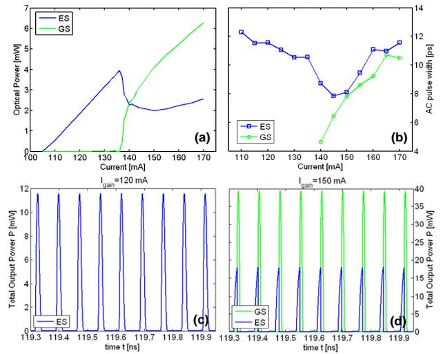
Figure 1. (a) GS and ES average output power versus injected current in the gain section at 0 V SA bias; (b) ML autocorrelation pulse width for GS and ES pulses versus the injected current in the gain section; (c) time trace of ES pulses at 120 mA; (d) time trace of GS and ES ML pulses at 150 mA.
