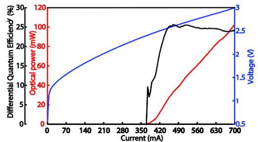
Figure 3. L-I-V curves from an EP-VECSEL with a disc contact  $\varnothing$  of 140  $\mu\text{m}$ , top contact  $\varnothing$  of 300  $\mu\text{m}$  and using a 5% output coupler.
