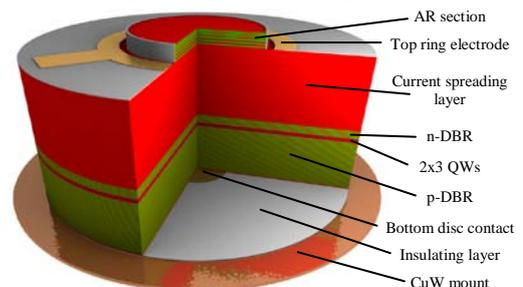
Figure 1. Sketch of our EP-VECSEL gain structure.
