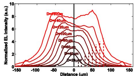
Figure 4. Electroluminescence profiles of EP-VECSELs with different back contact diameters recorded at high current injection.
