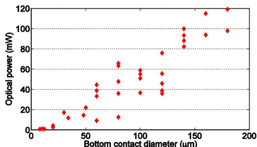
Figure 2. Output power of EP-VECSELs in a straight cavity with a 10% output coupler as function of the bottom disc contact diameter.
